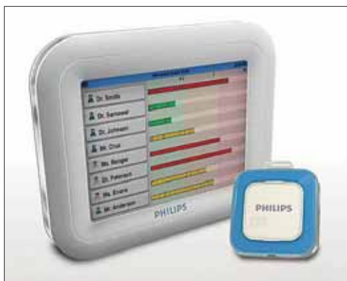
Physicians exposed to radiation on a daily basis have long been concerned about minimizing the risk. Researchers in Spain evaluated the new Philips Healthcare occupational Dose Aware System (DAS) showing staff radiation doses in real time. Dosimeters ( bottom ) worn by healthcare staff members ( left, right ), wirelessly track radiation levels every second and relay them to a base-station screen mounted close to the diagnostic monitors, providing an opportunity to improve personal protection
